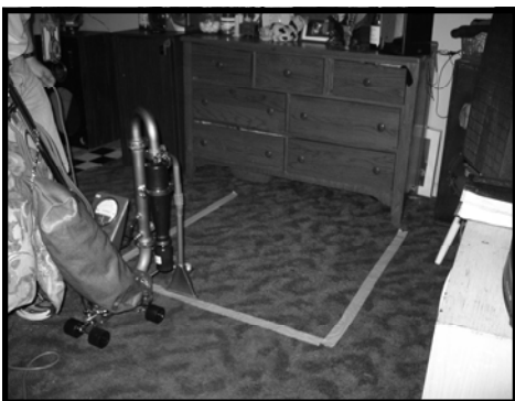
Special vacuum for dust sampling, with 1 square meter marked off for sampling.
