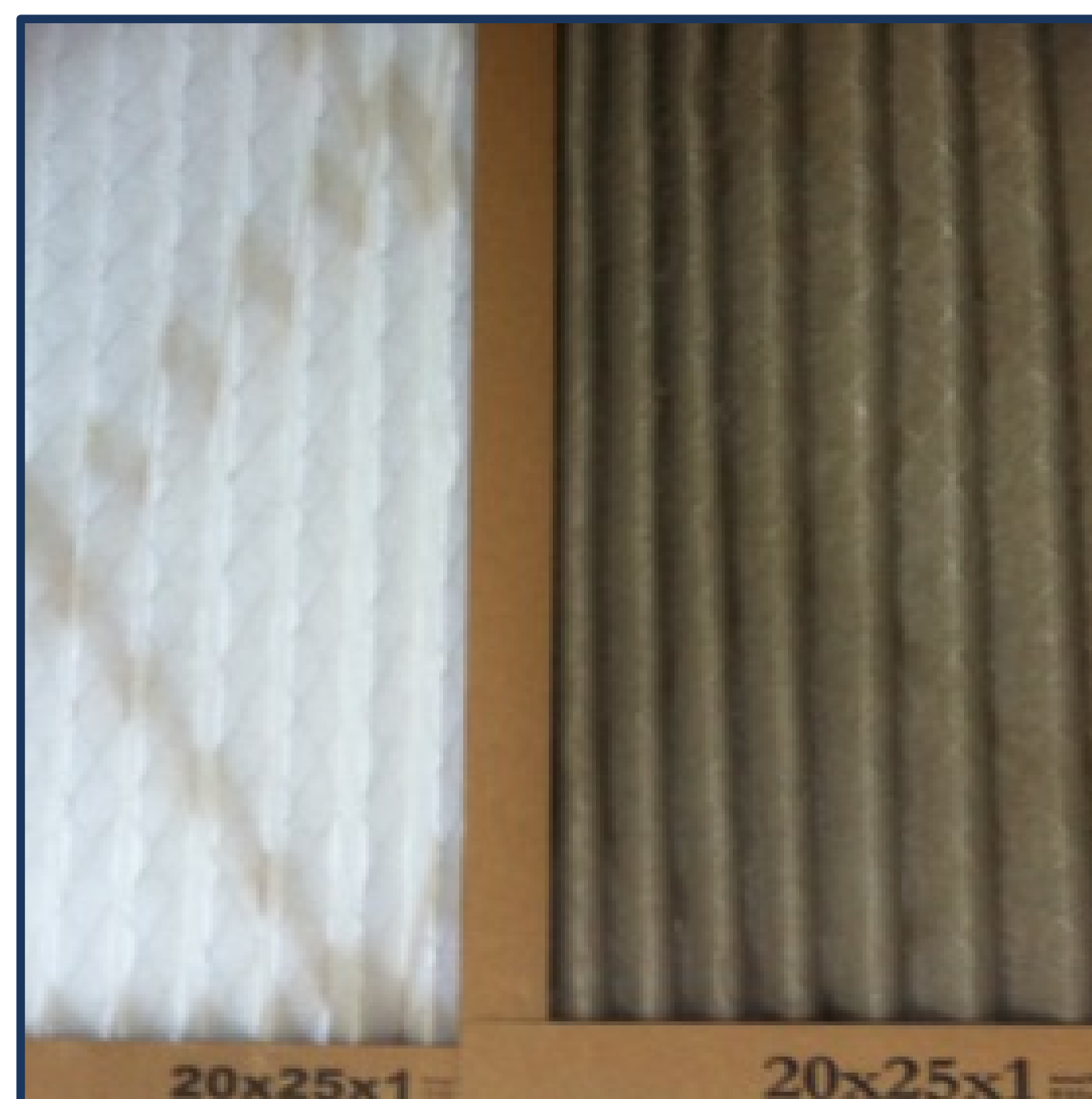
Replacing dirty air filters on a regular basis will improve indoor air quality.
