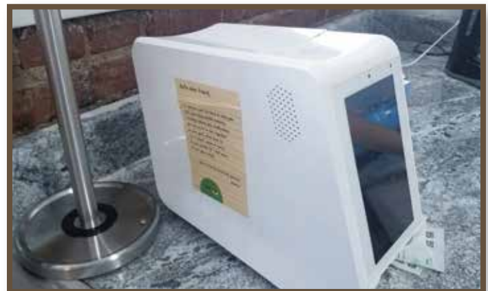
This programmable medications dispenser alerts the person who lives here about when it's time to take meds. The alerts increase in intensity until the meds are dispensed.
