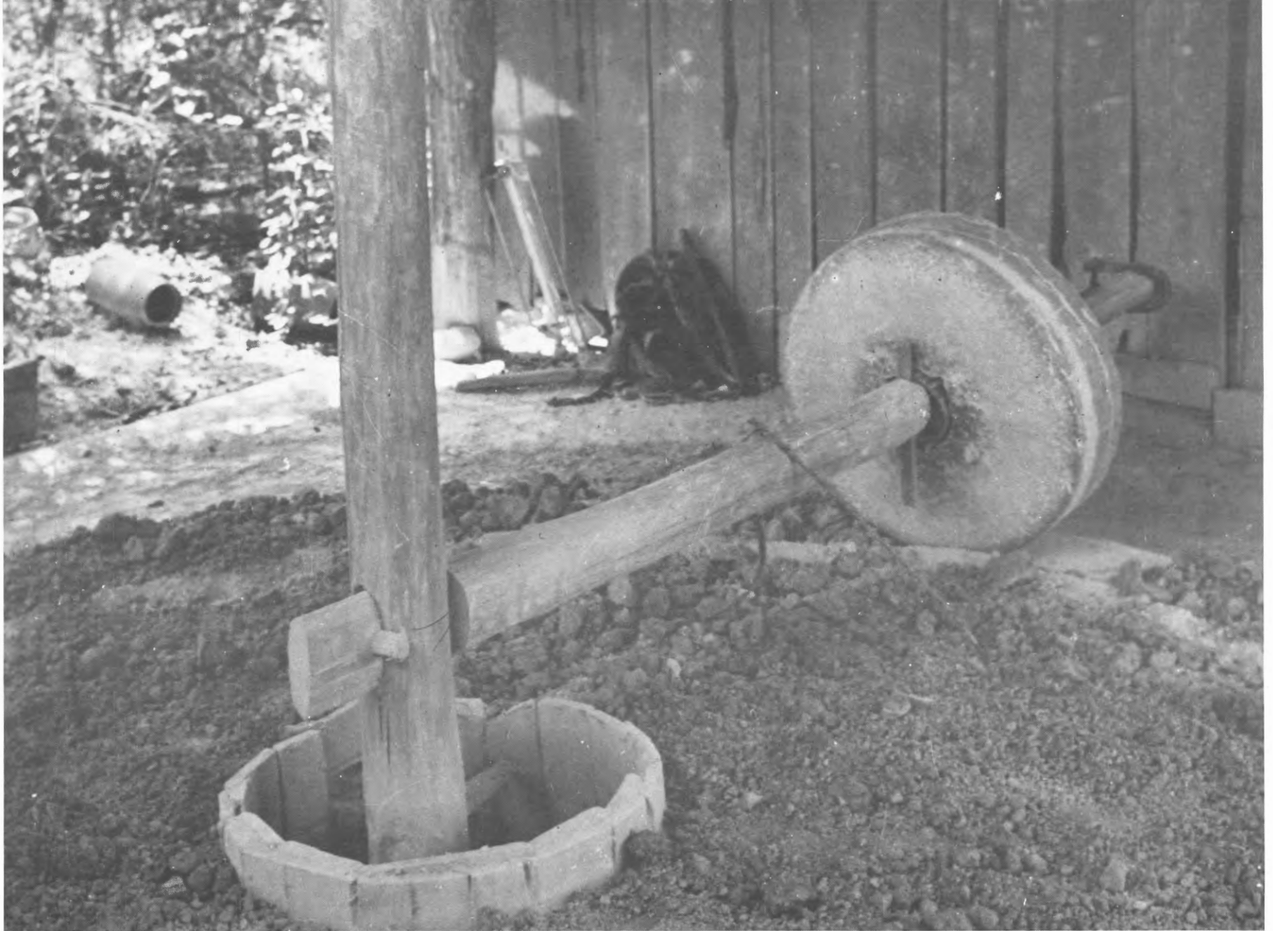
Figure 14. Photograph of clay mill at Eli LaFever pottery (40PM49) taken in 1936 or 1937. Photograph courtesy of Dillard Jacobs.
