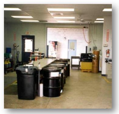
Picture 2: Proper drum segregation and labeling.
