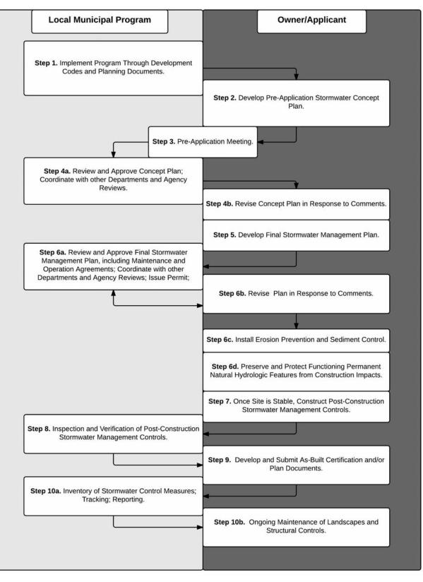
Figure 2.5: Typical Compliance Pathway for Permanent Stormwater Runoff Management for New Development and Redevelopment Projects.
