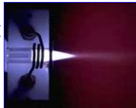
Samples are decomposed to neutral elements in a high temperature argon plasma (pictured above) and analyzed based on their mass to charge ratios.
