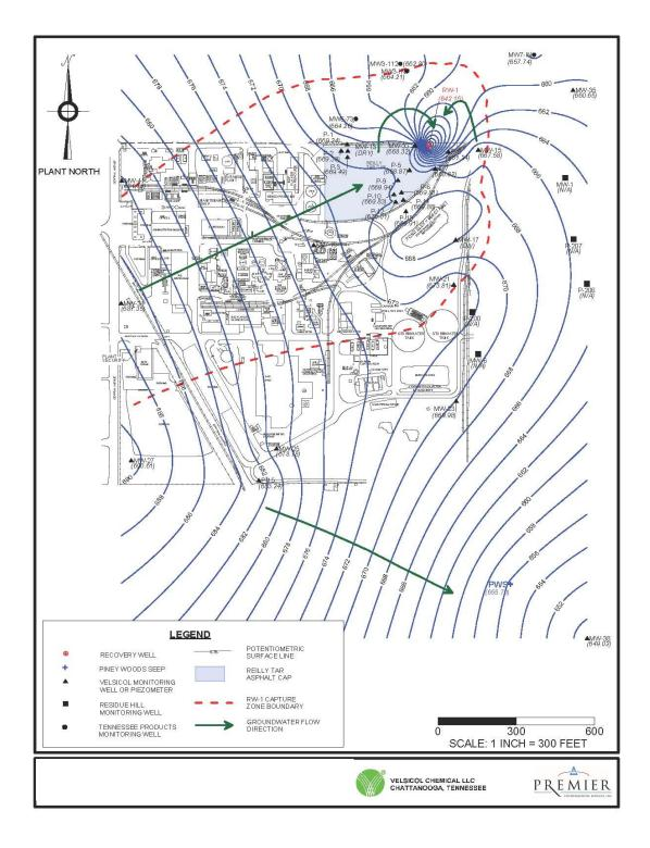
**Figure 5.** Bedrock interval groundwater surface map for the Velsicol Site. Like the groundwater in the soil interval, the groundwater in the bedrock also moves to well RW-1 and to Piney Woods Spring. Source: MEC 2011.
