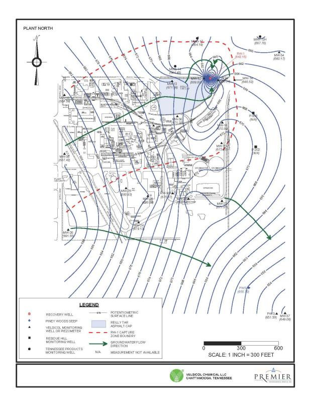
**Figure 4.** Soil interval groundwater surface map for the Velsicol Site. Groundwater flows to well RW-1 and Piney Woods Spring. Source: MEC 2011.
