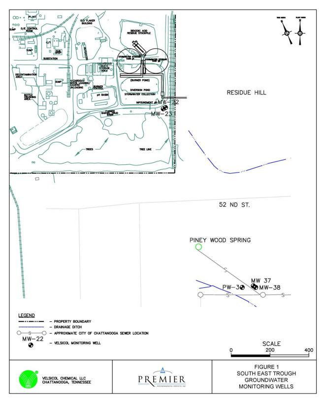
**Figure 7.** View showing the southeastern portion of the Velsicol Site and the locations of Residue Hill and Piney Woods Spring. The figure also shows the groundwater monitoring wells for the southeastern portion of the Velsicol Site and Piney Woods Spring are located. Source: MEC 2011.
