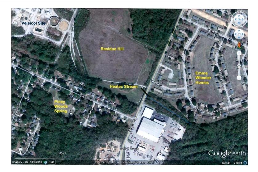
**Figure 6**. Location of Heatec stream where sediment samples were collected as part of the Velsicol Site investigation. Note the relation of the stream with the Velsicol and Residue Hill Sites. Chemicals found in the stream may be from either site. Source: Google Earth.
