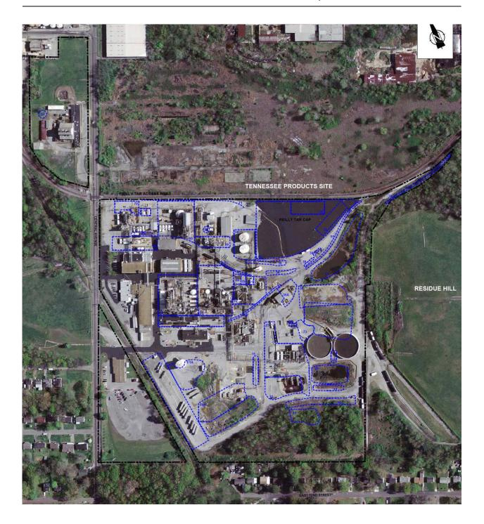
**Figure 2.** Aerial view of Velsicol Chemical Company Site, Alton Park, Chattanooga, TN. Black dashed and dotted line is the limits of the Velsicol property. Blue forms represent the outlines of solid waste management units (SWMUs). Only two onsite buildings remain. One surface water containment structure also remains. Most of the buildings and process equipment were removed during 2007 and 2008 with only concrete building floor slabs remaining from those buildings. Source: MEC 2011.
