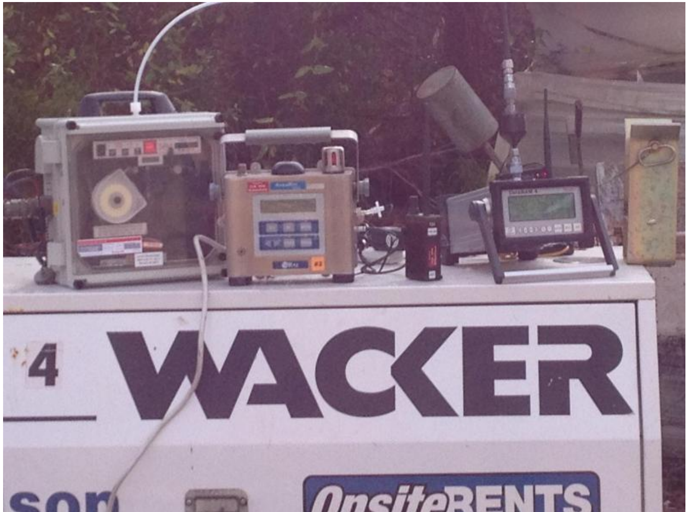
Air monitoring instrumentation near the fire that was used to measure air quality, such as volatile organic compounds, chlorine, hydrochloric acid, phosgene, and carbon monoxide, from December 18 through December 20, 2013. Source: EPA.
