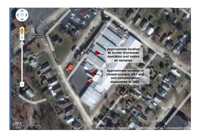
FIGURE 2 - Indoor air sampling locations inside the former drycleaning area at the Rental Uniform Company. Recreated from Figure 1 in the Indoor Air Sampling Report prepared by S&ME dated February 2010.
