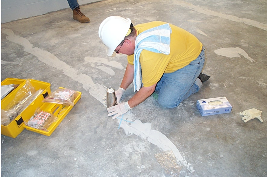
Photo of Emflux sampling over patched concrete floor at Downtown School Memphis, Shelby County, Tennessee (Photo credit: Shanna Davis, PEI)
