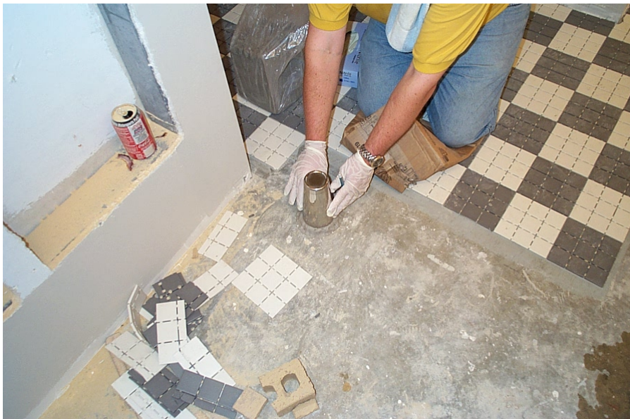
Photo of Emflux sampling near tiled-floor at Downtown School Memphis, Shelby County, Tennessee (Photo credit: Shanna Davis, PEI)
