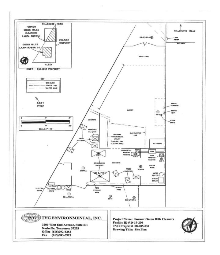
**FIGURE 3** - Details of the Former Green Hills Cleaners Lease Space. Drawing Credit: TVG Environmental Inc., Phase 1 Solvent Impact Assessment, September 15, 2008.
