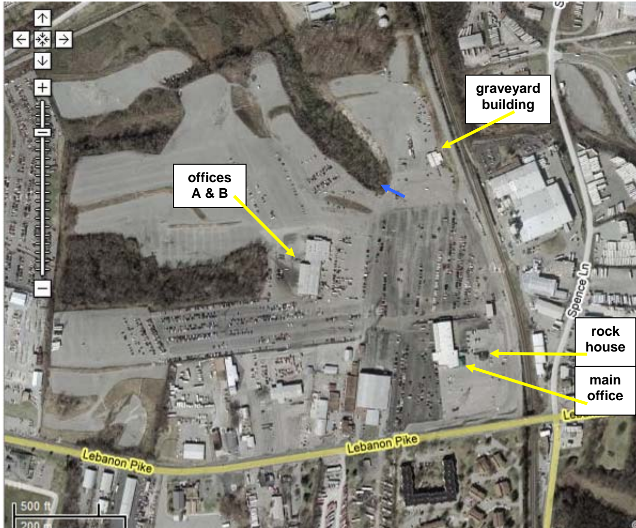
FIGURE 1. Aerial image showing the current Tennessee Auto Auction land use over the former Lebanon Road Landfill. The locations where methane gas levels have been measured in site reports have been noted. (Image credit: Google 2007)
