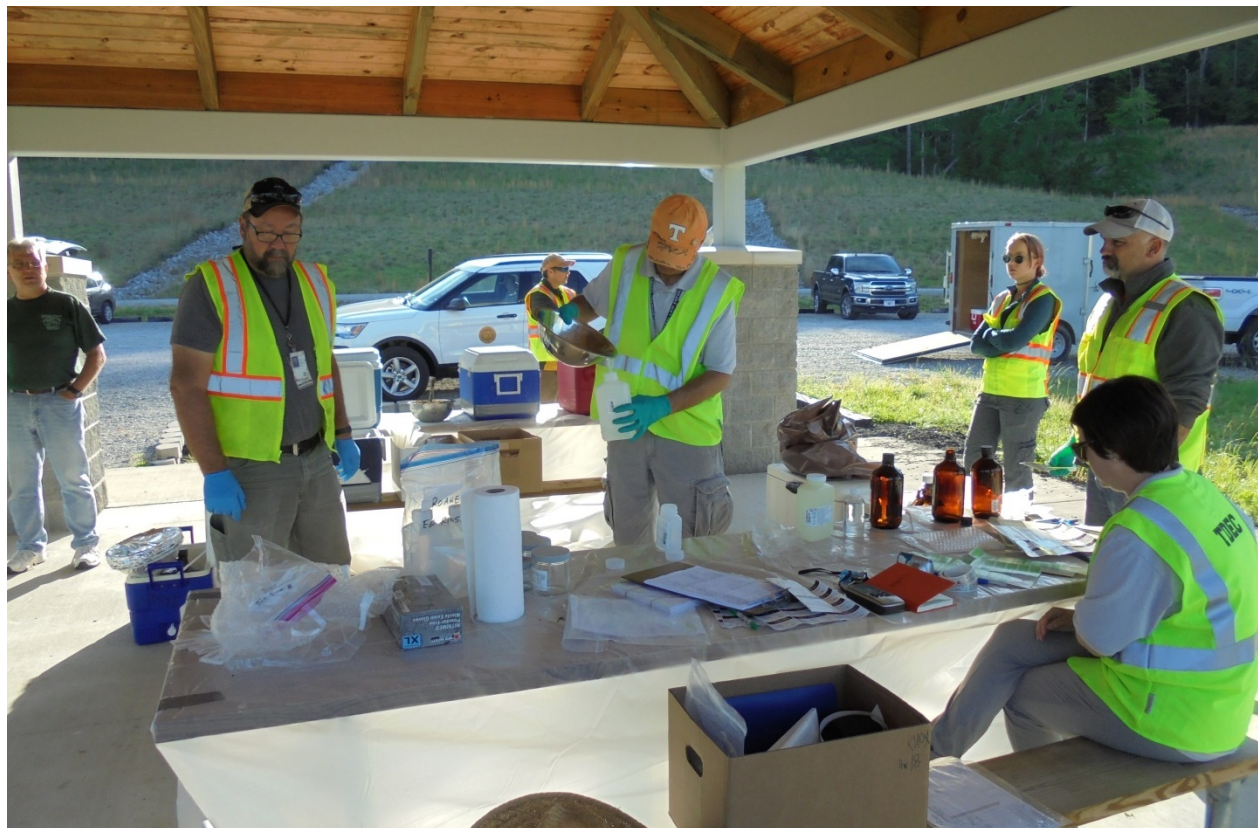
Photo 3. Tennessee Department of Environment and Conservation field sampling staff, TVA field sampling personnel, and a Roane County Environmental Review Board representative look on as an equipment field blank is collected from a sample collection and mixing bowl at the sample management station set up in the onsite pavilion (Source: TDH, May 7, 2019).
