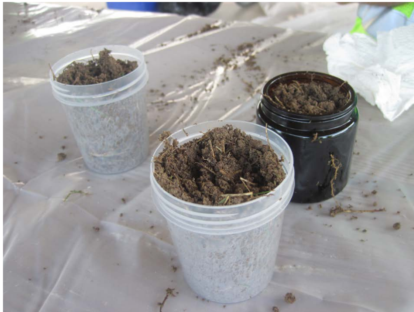
Photo 6. Samples in lab analysis jars during sample splitting with TVA. Each sample was sent for analysis of the following contaminants- metals, Radium 226 and 228, fluoride, sulfide and chloride and Polarized Light Microscopy (PLM). Photo taken Monday, May 6, 2019.
