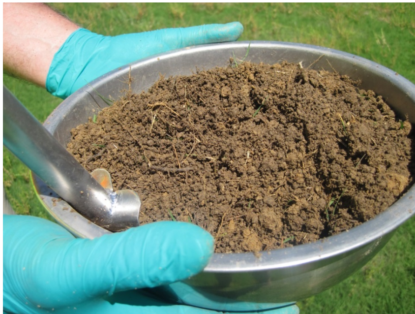
Photo 3. Bowl following collection and homogenization of 9-point composite sample # 1. Photo taken on Monday, May 6, 2019.
