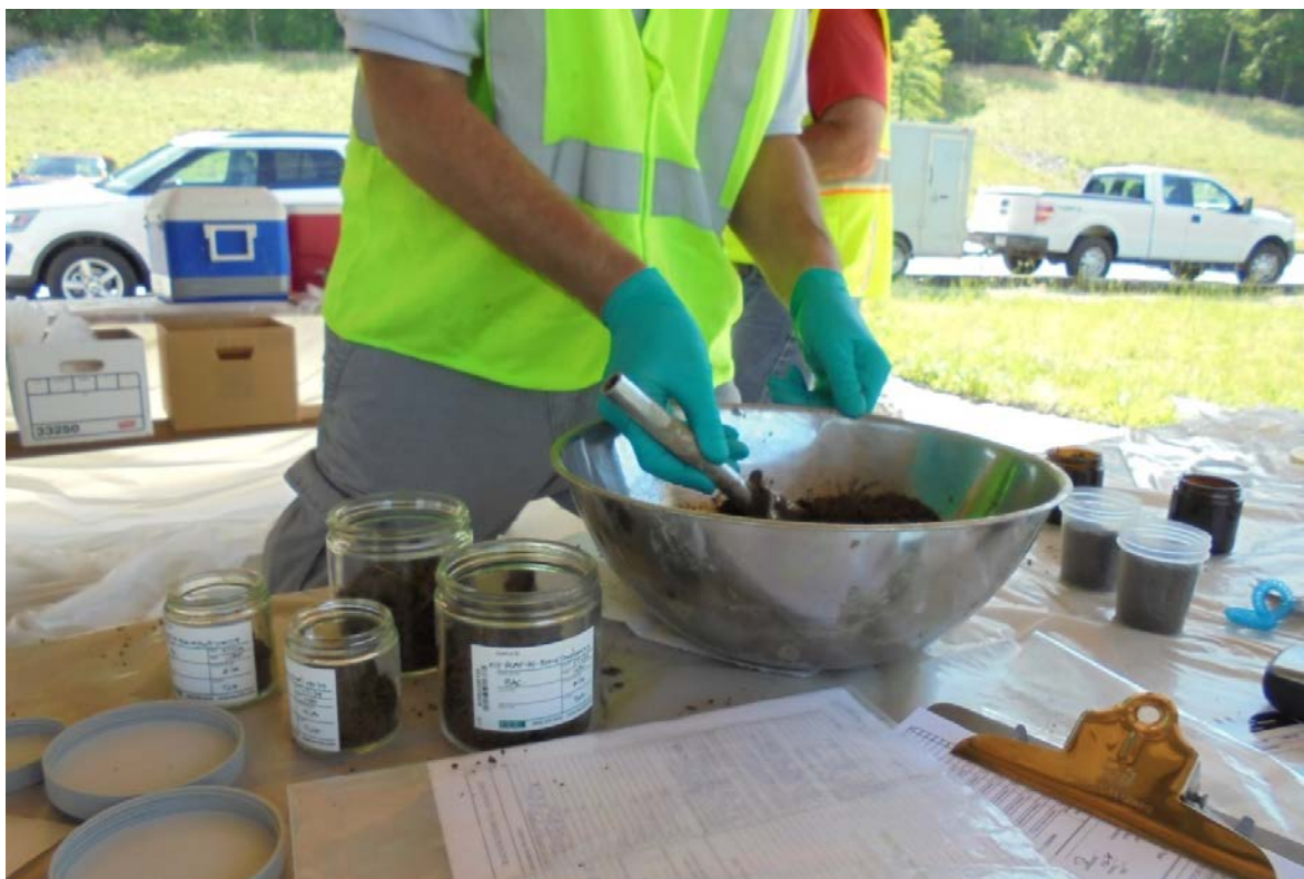
Photo 6. A Tennessee Department of Environment and Conservation geologist mixes the 9 sub-samples at the sample management station in the sports complex pavilion before placing the soil in laboratory-supplied sample containers (Source: TDH, May 7, 2019).
