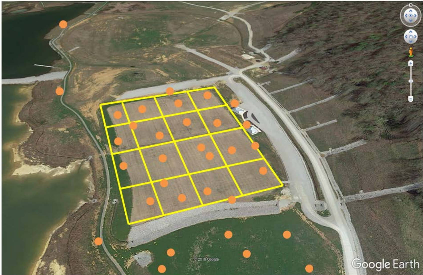
Figure 5. Orange dots represent approximate suggested surface soil sampling locations for Athletic Fields, Festival Field, and Walking Trail to ensure areas are safe for public recreational use. Image source: Google Earth 2019
