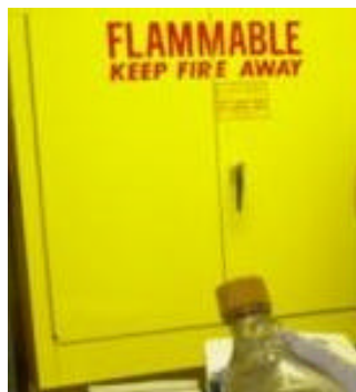
A Flammable Chemicals storage cabinet helps achieve long-term responsible chemical management. Photo courtesy of TDEC.
