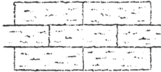
Figure 7-7.10-1. Correct sod placement
