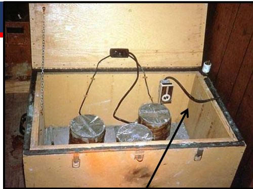
Storage for initial curing of concrete cylinders
