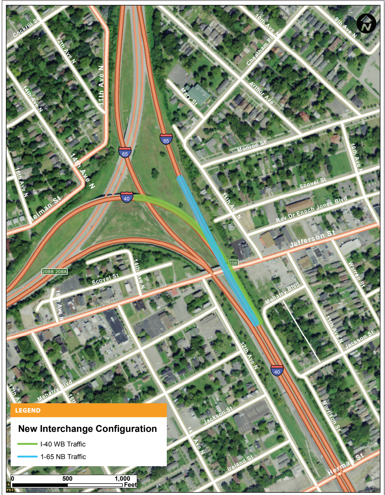
Figure 4-6. New I-40/I-65 Interchange Configuration
