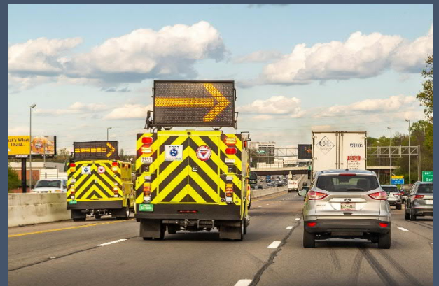
TDOT's HELP patrol assists motorists and law enforcement to clear travel lanes quickly when incidents occur in major urban areas. Extending some version of this service to the entire corridor would improve traveler safety, both for motorists who are affected directly and for those traveling around them.
