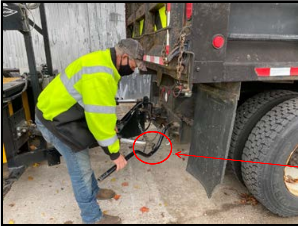
Photo D – Cylinder removed from cradle and placed onto the pin near the center of the tool.
