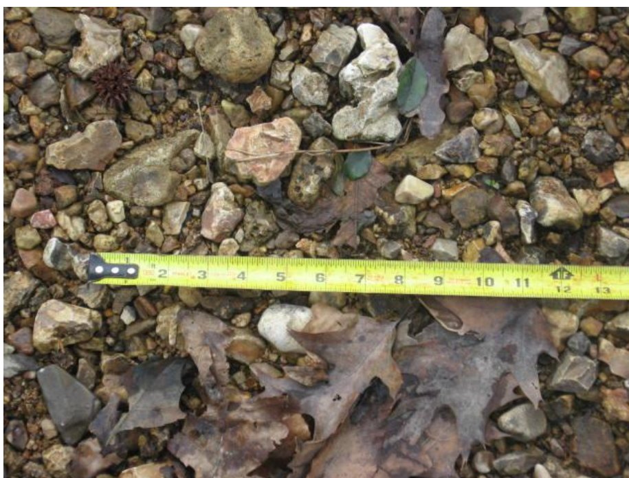
Figure 11A-5 Typical Sample of Wash Load Location: Furnace Branch, Wayne County, Tennessee (2010)
