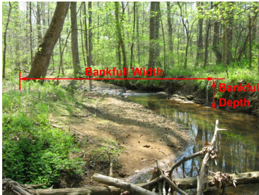
Figure 11-10 Stream with Bankfull Width and Depth Shown Location: Sulphur Branch, Overton County, Tennessee (2010)
