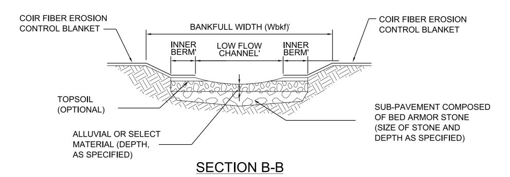
CONSTRUCTED ALLUVIAL RIFFLE
