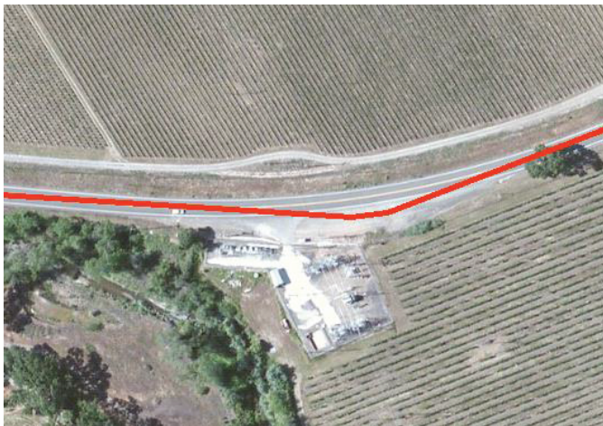
Figure 20. Example of horizontal curve realignment (39).
