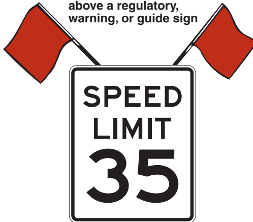
Figure 2A-1. Examples of Enhanced Conspicuity for Signs
