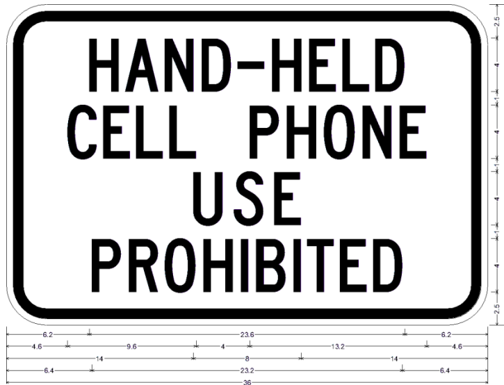
3.0" Radius, 0.8" Border, 0.5" Indent, Black on White; *HAND-HELD* C 70% spacing; *CELL PHONE* C 70% spacing; *USE* C; *PROHIBITED* C 70% spacing;
