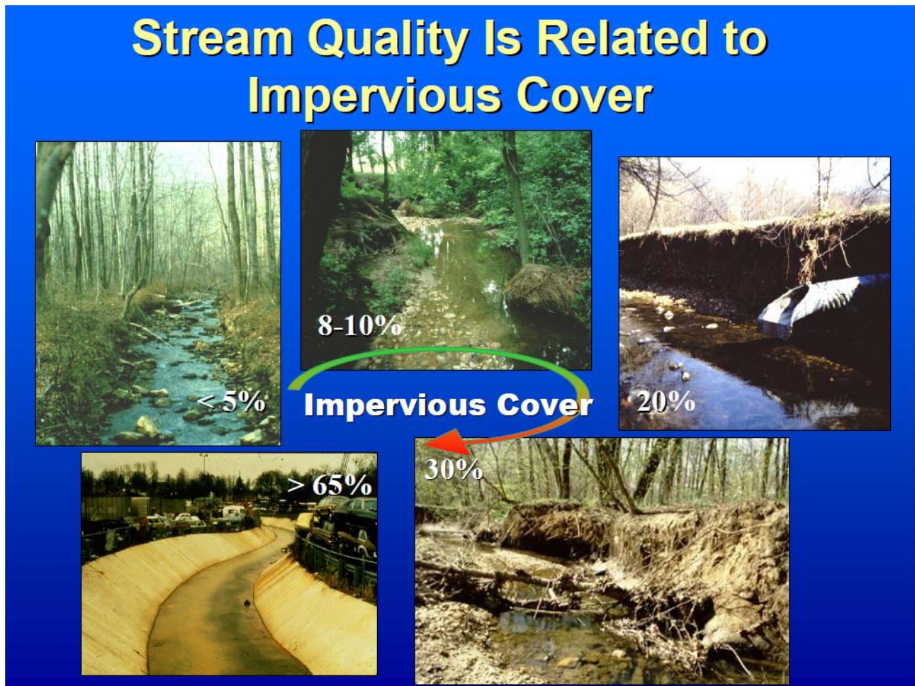
Figure 32. Effect of Impervious Cover in the Upstream Watershed
