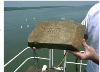
Fire bricks helped protect wood steamboats from the heat of the steam boilers. The stamped maker's marks help archaeologists identify the vessels.
