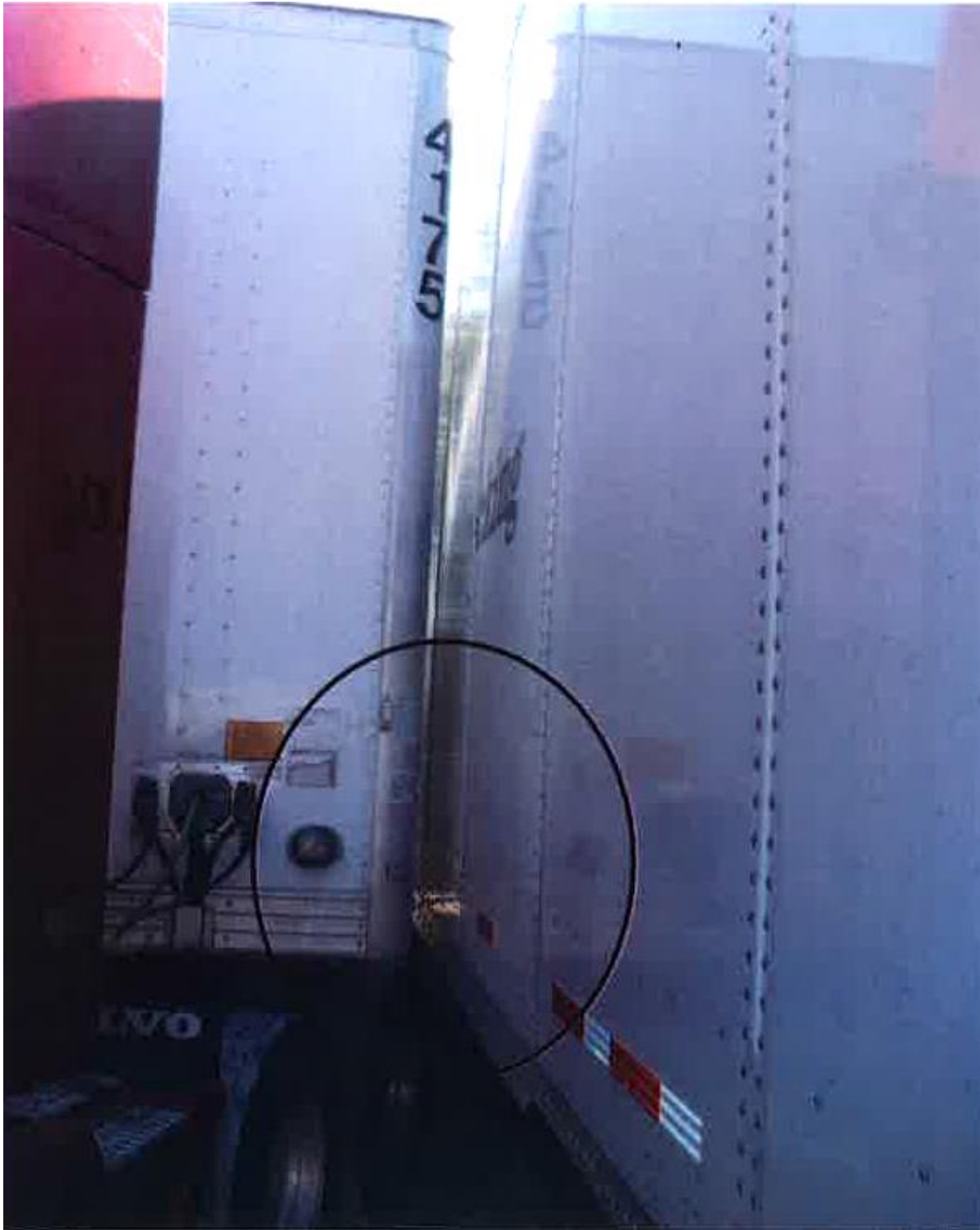
Photo 2 of 3 – The circle denotes the area where the victim was crushed and measured approximately 4/12 to 5 inches between the two trailers.
