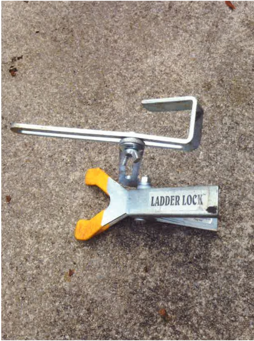
Photo 2 of 2 – The photo shows a similar ladder lock that comes equipped on all Directv work vans.
