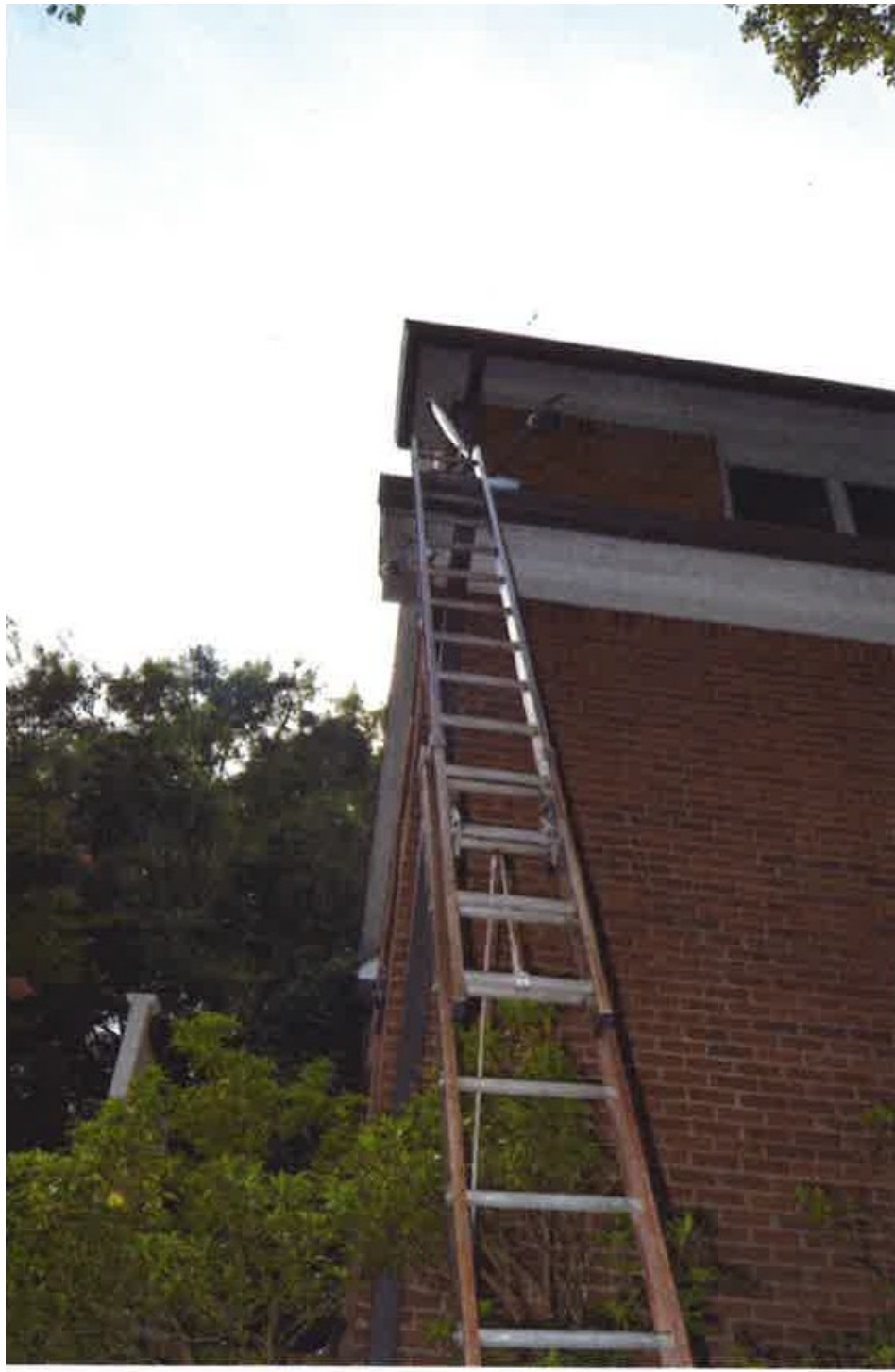
Photo 1 of 2: Photo shows the 28 foot extension ladder against the residential home. The height of the roof was measured 20 feet
