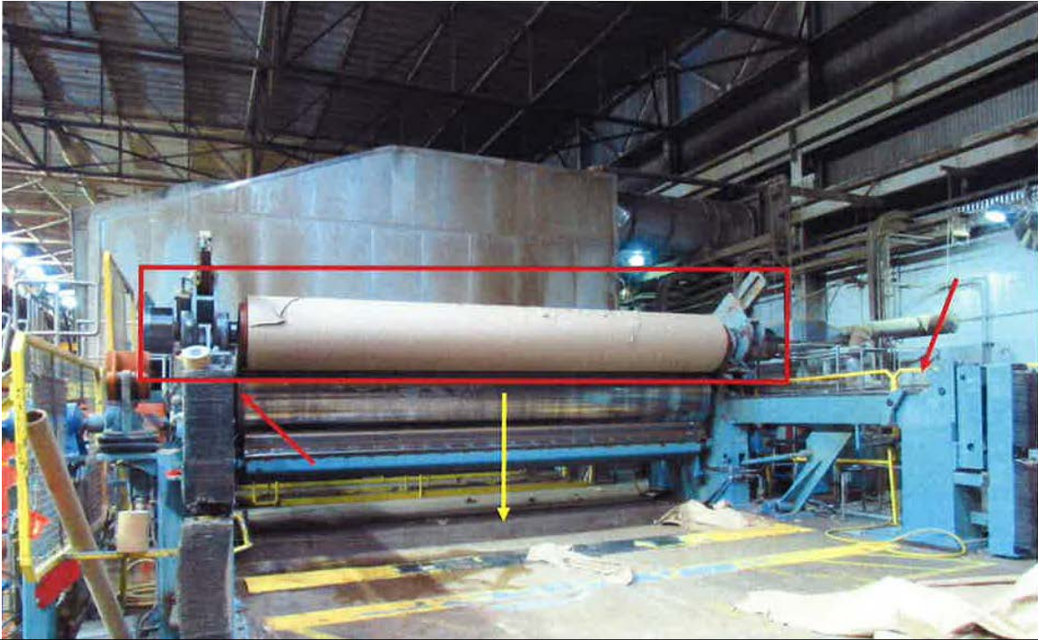
Photo 1 of 2 – The parent reel where the “snap off” occurred is located in the primary arms designated by the red square. The reel that had just finished was sitting on the frame rails designated by the red arrows. The yellow arrow designates a fall hazard where scrap paper would be removed by a moving conveyor located below the machine.
