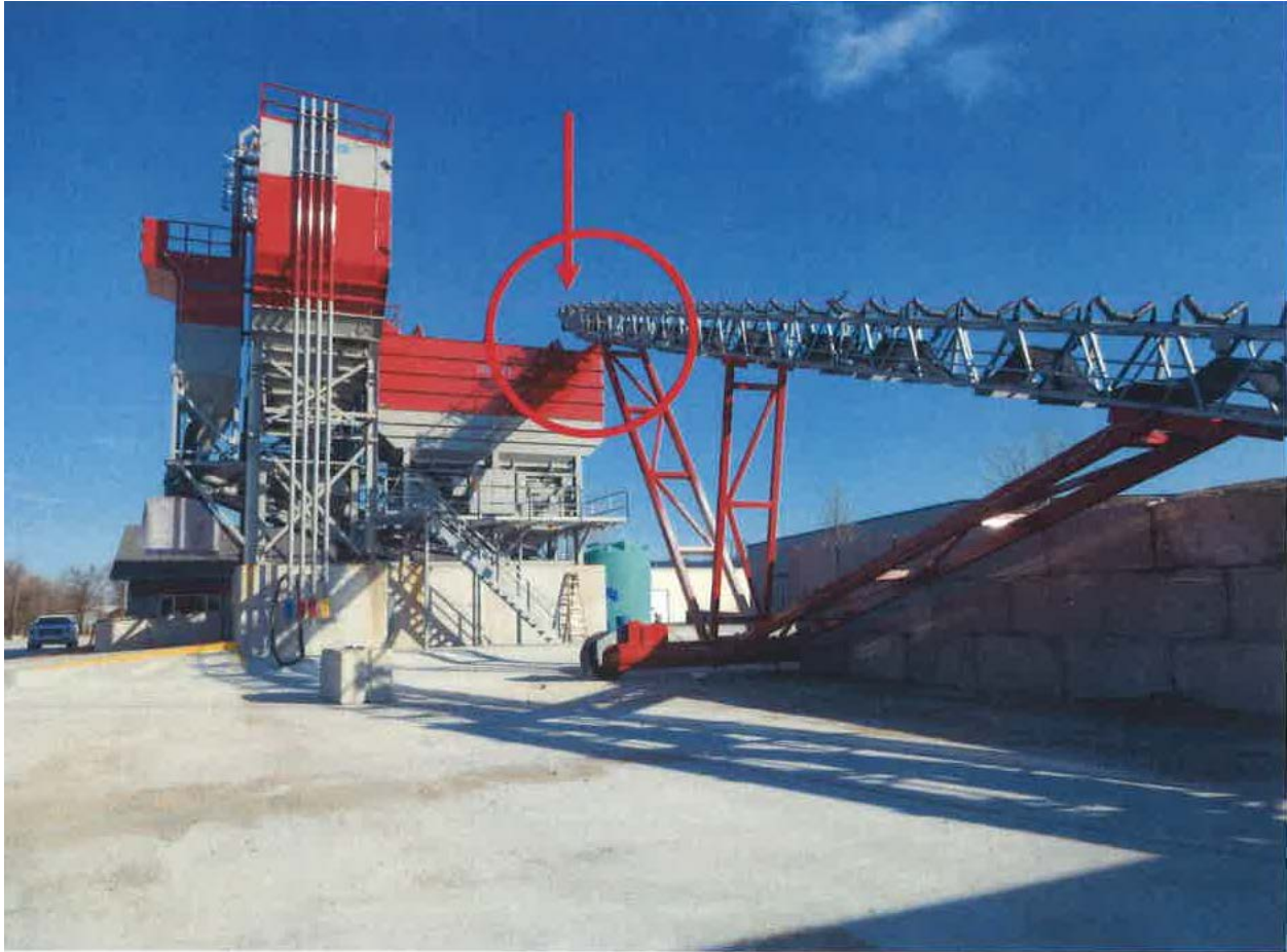
Photo 1 of 2 – The red arrow and circle indicates where the incident occurred along the 125' x 10" aggregate conveyor located behind the batch plant.
