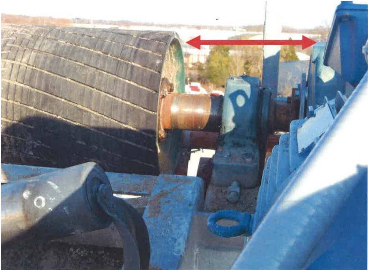
Photo 2 of 2 – The red arrow indicates the area where the victim was pulled into the machine at the head pulley and frame of the 125' x 10" aggregate conveyor.
