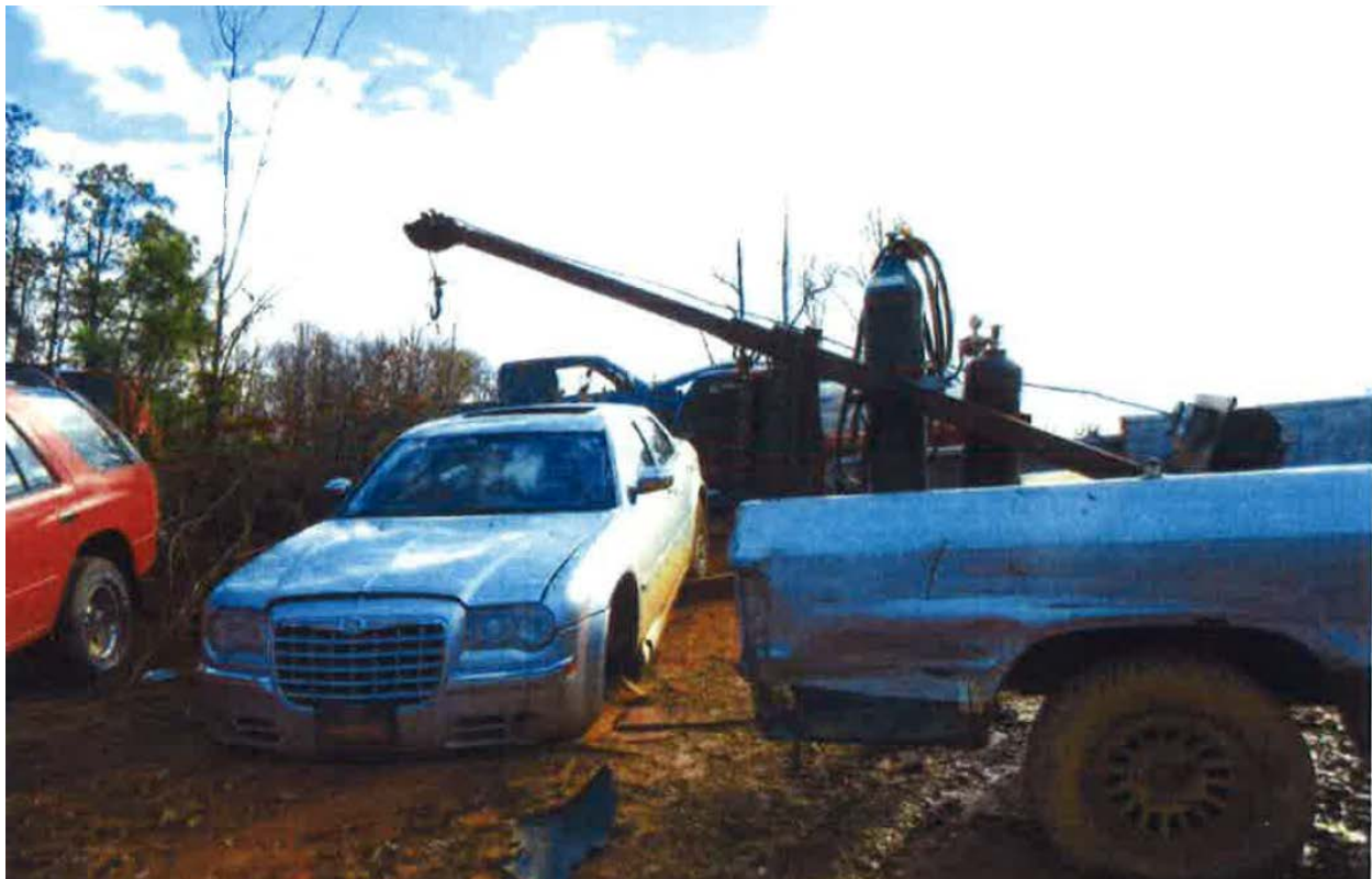
Photo 1 of 1 – Shows the two vehicles involved in the incident. The car was hoisted off the ground by the hoisting device in the bed of the truck.
