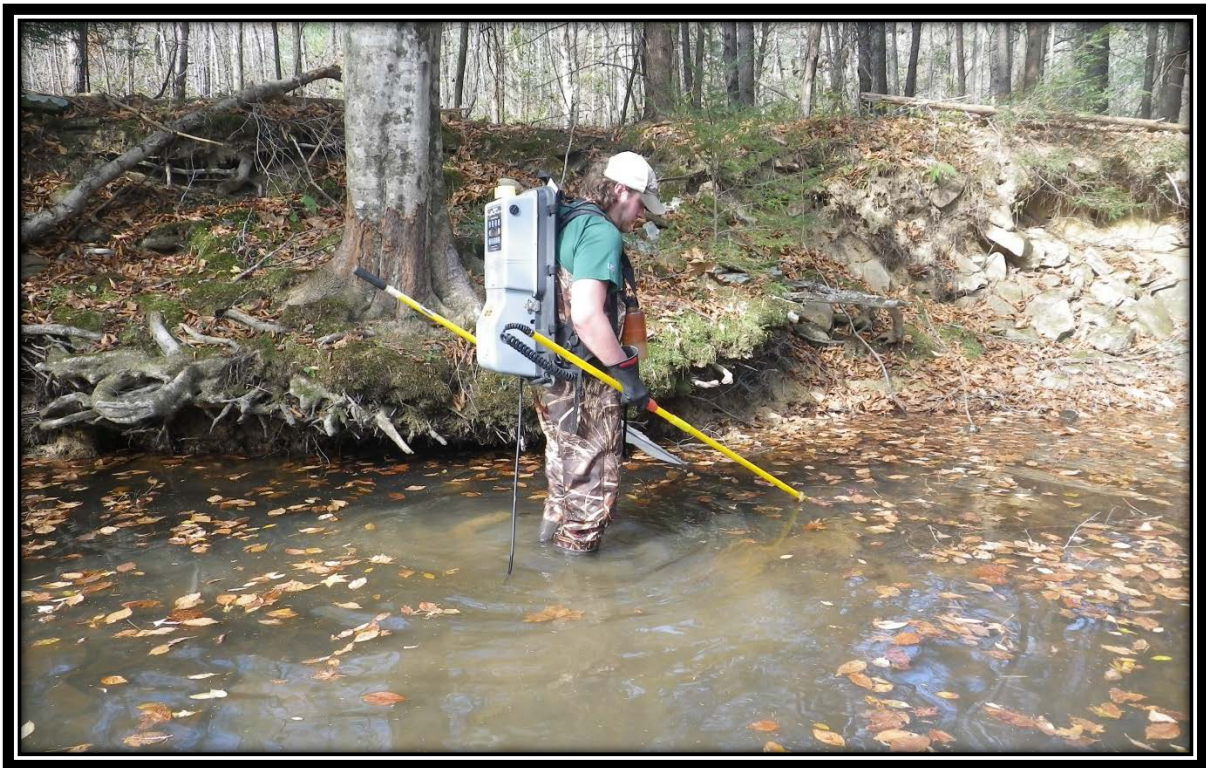
Marka Smith electroshocking in Brimstone Creek in Scott County to collect fish for tissue analyses. Photo provided by Carrie Perry, Aquatic Biology Section, TDH.
