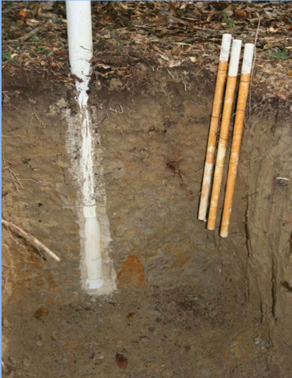
Monitoring well and IRIS tube soil hydrology study NRCS study site, Coffee County, Tennessee
