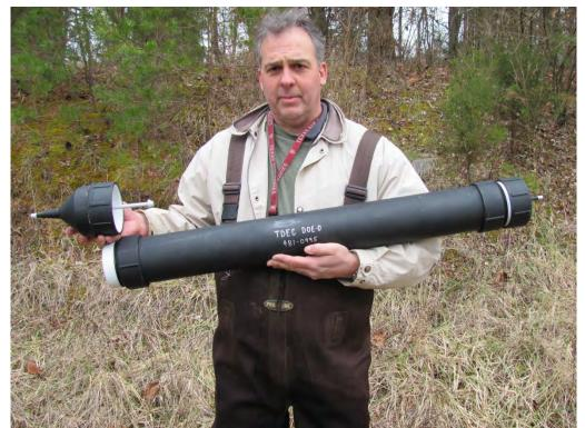
**Figure 3: Photo of Sediment Trap**
