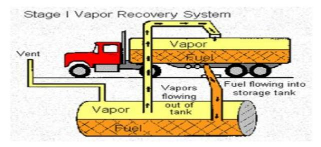
Stage I Vapor Recovery Systems are designed to capture the vapors that pushed out of the tank when the cargo truck is filling the storage tank. These vapors are pulled into the cargo truck where they can later be condensed back into liquid fuel. The Stage I Vapor Recovery System in this way helps lessen the release of gasoline vapors and enables the recovery of gasoline that has become a vapor. The illustration above shows the basic operation of a dual-point Vapor Recovery system.
