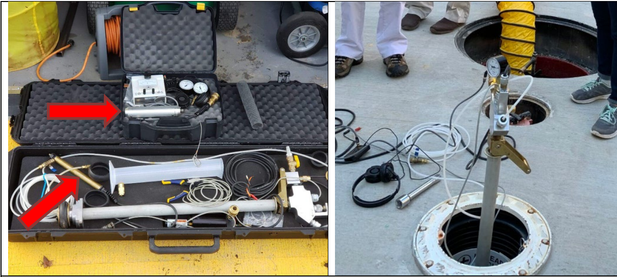
Mesa Engineering's 2-D testing equipment pictured above. Notice the sonde (top arrow) and water sensor (bottom arrow) in the top left photo.
