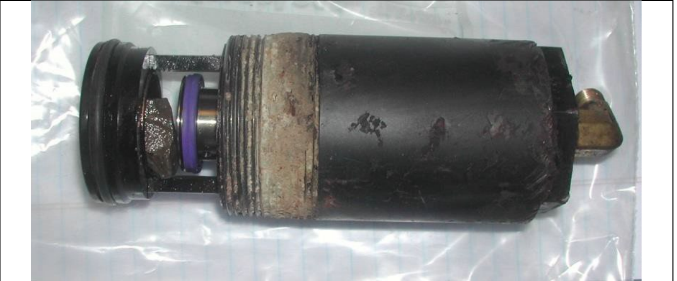
Rock inserted to disable line leak detector
