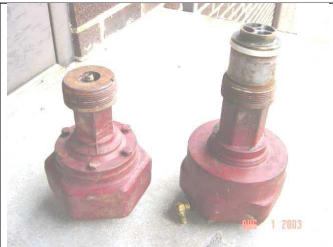
Red Jacket DLD with intake screen and metering pin removed on left
