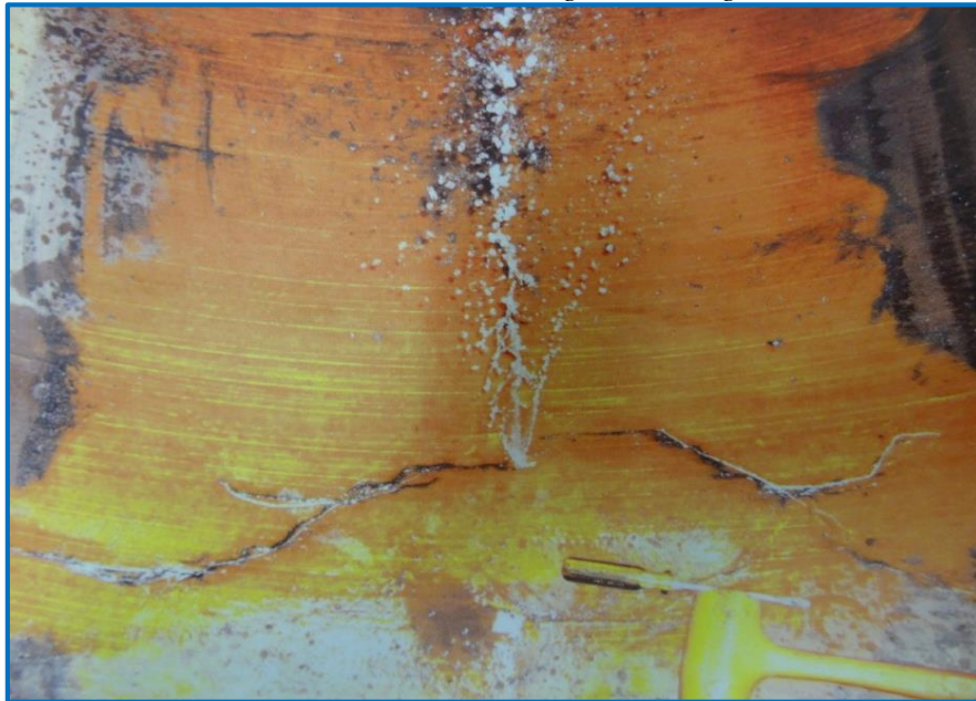
92 Octane UST interior – water entering tank through crack
