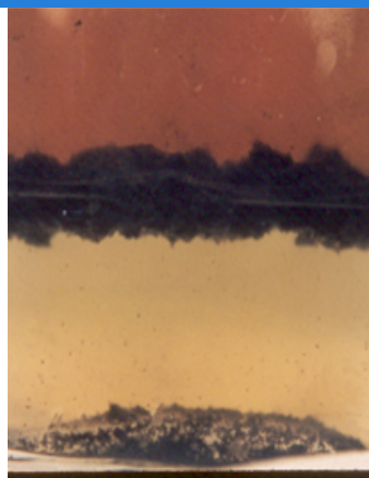
F2. - Diesel Tank Bottom Sample w Microbes
