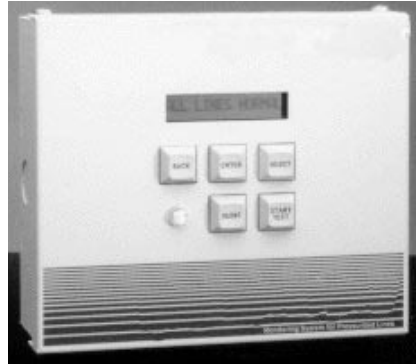
Figure 14 - An Example of an ELLD Control Panel
