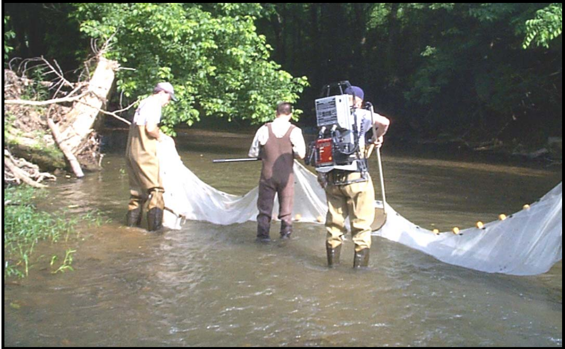
Fish can be collected for analysis with the use of a backpack shocker. Photo provided by Jonathan Burr, Knoxville OFFICE.
