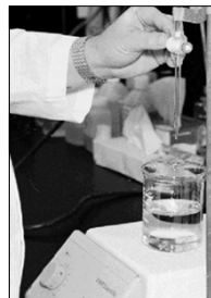
Titrate with 0.025M sodium thiosulfate. Titrate until a pale straw color.
