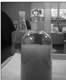
After addition of reagents, a manganese hydroxide floc appears if oxygen is present.
