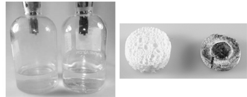
Figure 6. The calibration bottle on the right is clean. The calibration bottle on the left actually has algae growing in it which could affect the calibration values.
