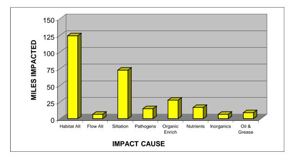
*Figure 3-9. Total Impacted Miles by Cause in the Stones River Watershed.* Data are based on Year 2000 Water Quality Assessment.
