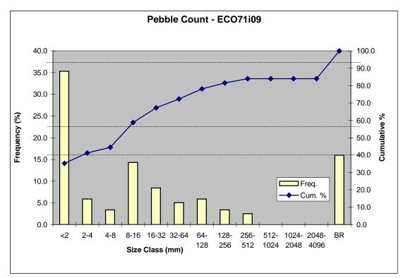
Figure 3-17a. Particle Count Histogram and Cummulative Frequencey Plot for West Fork Stones River Fluvial Sampling Site (River Mile 32.3). BR, Bed Rock. Data were collected on October 1,1997.
