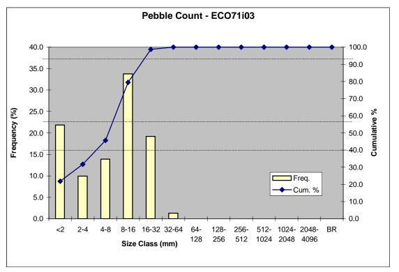
Figure 3-18. Particle Count Histogram and Cummulative Frequencey Plot for Stewart Creek Fluvial Sampling Site (River Mile 16.7). BR, Bed Rock. Data were collected on October 1,1997.
