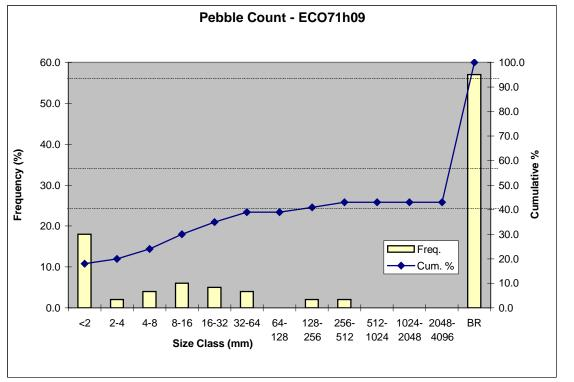
Figure 3-16b. Particle Count Histogram and Cummulative Frequencey Plot for Carson Fork Fluvial Sampling Site (River Mile 5.4). BR, Bed Rock. Data were collected on June 11,1999.
