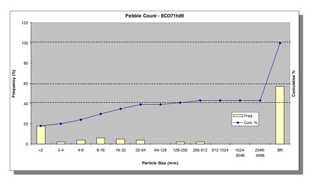
Figure 3-12. Particle Count Histogram and Cummulative Frequency Plot for West Fork Stones River Ecoregion Reference Site.
