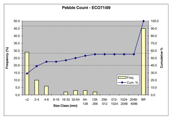
Figure 3-17c. Particle Count Histogram and Cummulative Frequencey Plot for West Fork Stones River Fluvial Sampling Site (River Mile 32.3). BR, Bed Rock. Data were collected on June 3, 1998.
