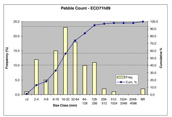
Figure 3-16a. Particle Count Histogram and Cummulative Frequencey Plot for Carson Fork Fluvial Sampling Site (River Mile 5.4). BR, Bed Rock. Data were collected on August 31,1998.
