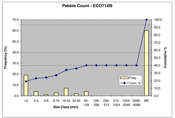
Figure 3-17b. Particle Count Histogram and Cummulative Frequencey Plot for West Fork Stones River Fluvial Sampling Site (River Mile 32.3). BR, Bed Rock. Data were collected on September 1,1998.
