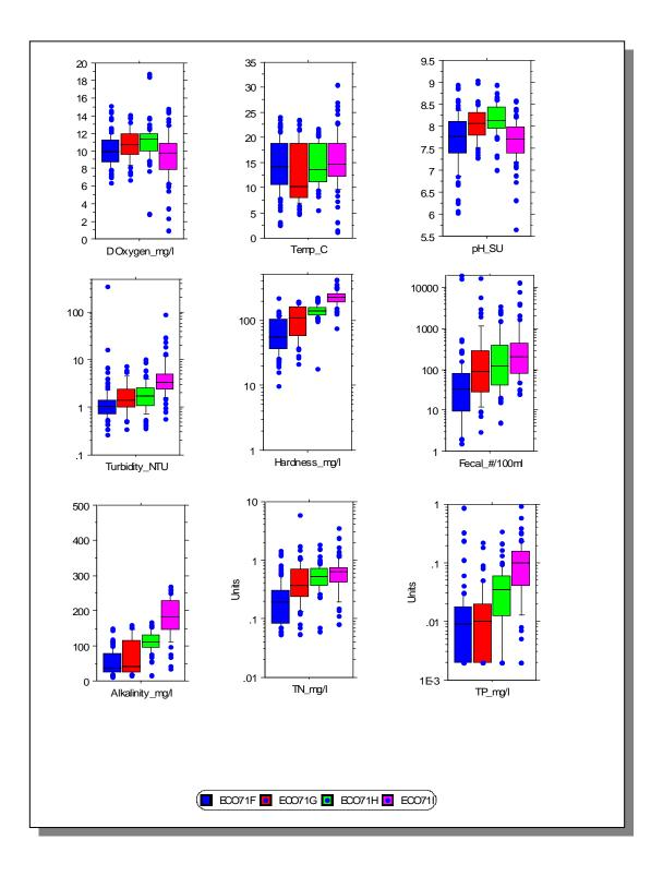
*Figure 3-4. Select Chemical Data Collected in Upper Duck River Watershed Ecoregion Sites.* Boxes and bars illustrate 10<sup>th</sup>, 25<sup>th</sup>, median, 75<sup>th</sup>, and 90<sup>th</sup> percentiles. Extreme values are also shown as dots. Fecal, fecal coliform bacteria; TN, Total Nitrogen; TP, Total Phosphorus.
