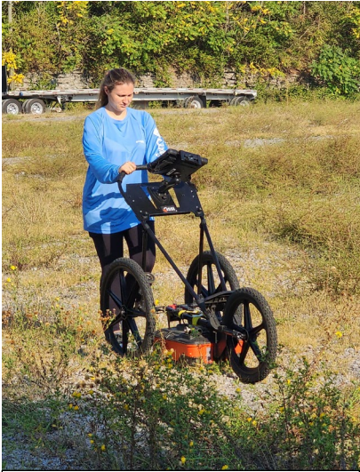
Vanderbilt Graduate Student Conducting GPR at Fort Negley
