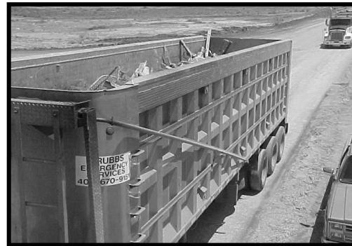
Figure 11.3 - Less Than 100% Loaded Truck
