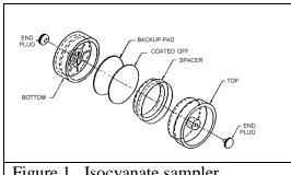
Figure 1. Isocyanate sampler.
