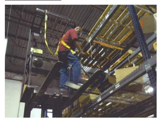
Photo 1 of 2 – Crown order picker powered industrial truck (PIT).
