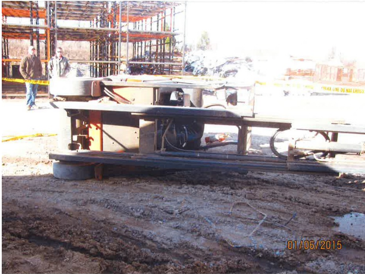
Photo 2 of 2 – Forklift on its side with the attachment in the raised position
