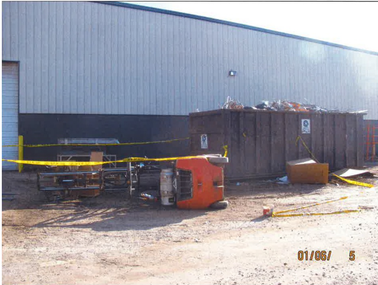
Photo 1 of 2 – Forklift on its side with the attachment in the raised position
