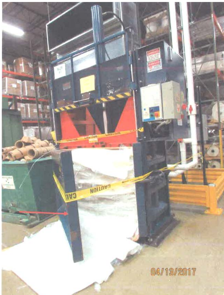
Photo 1 of 1 – The chamber door (red arrow) stuck the victim’s head when a walk behind forklift was used to force the door shut.
